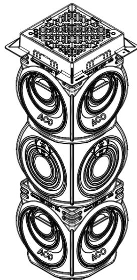
ISOMETRIC VIEW OUTLET/INLET/SILT CHAMBER
