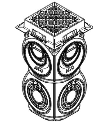
ISOMETRIC VIEW OUTLET/INLET CHAMBER
